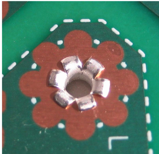
Eyelet/Pin after insert to PCB
